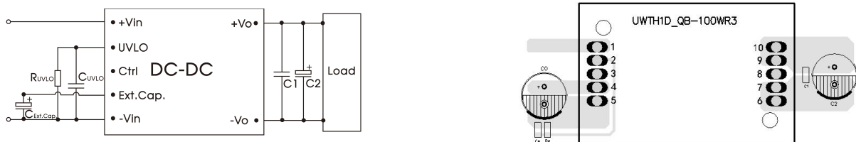
Fig.7 Recommended circuit and PCB layout for hold-up time
