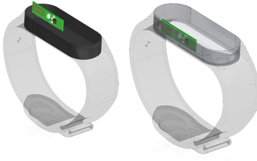
Figure 2.2: 3D representation of inductive force touch PCB showing orientation and detail
